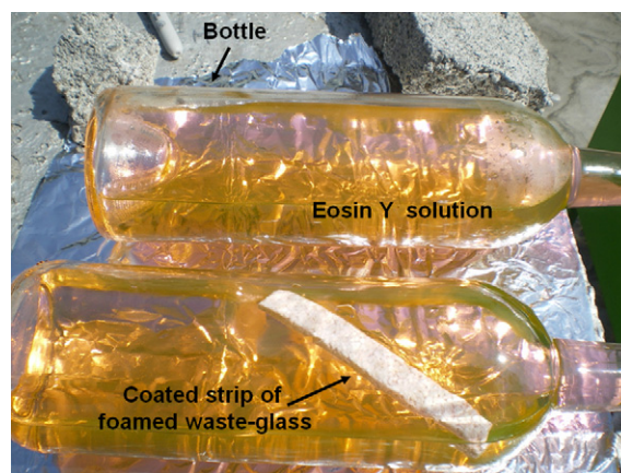
Fig. 2. Digital image during the course of solar photocatalytic degradation into a glass bottle of Eosin Y under irradiation of sunlight.
